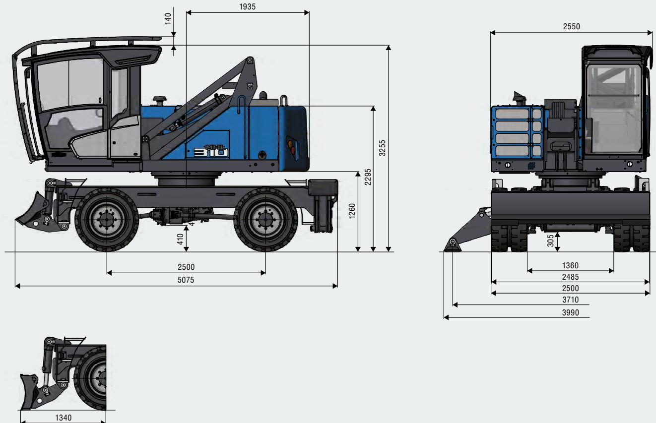
**TRANSPORT DIMENSIONS | TRANSPORTABMESSUNGEN | DIMENSIONS DE TRANSPORT [mm]**
